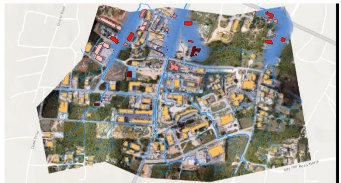
Figure 25 - Drainage Paths, Building Outlines and Highlights Buildings at Risk of Flooding
