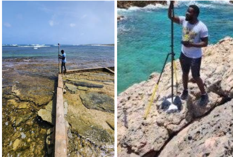
Figure 4 - GCPs in Anguilla using existing features (at left) and new targets (at right)
