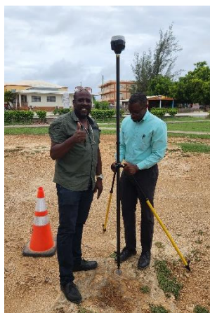
Figure 5 - Base Station on a known Control Point
