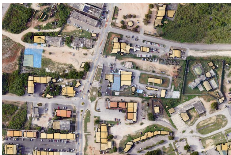
Figure 19 - Building Outlines Identified Using Machine Learning Models
